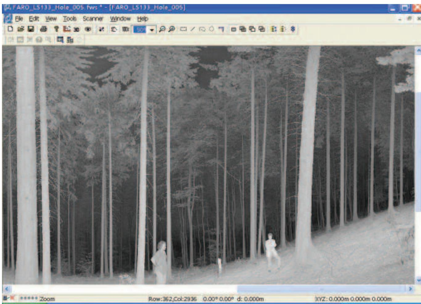
Figure 2: 3D image generated by the laser scanner.
